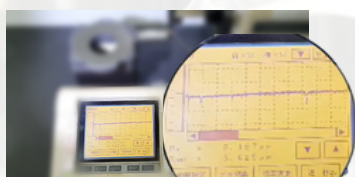
Surface roughness measurement Ra 0.187 µm
